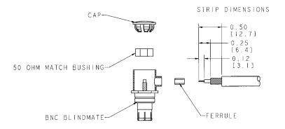
Figure 2-2. Blindmate Antenna Connector
